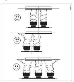
The cooker hood must cover the hob to ensure optimum extraction of cooking vapours:
